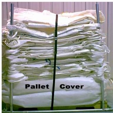
4. Once the frame is full, place securing strap over the stack and slowly apply tension, periodically push down the opposite side of the stack to help compress it evenly. Now the stack is stable and secure. Remove the four corner poles, place any extra strapping into the pallet cover.
